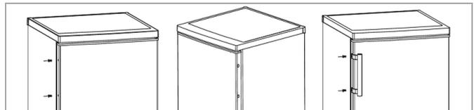
Remove the cover caps from the door outer side and tighten the handle with the delivered screws into the underlying holes. Put the included screw covers on.
