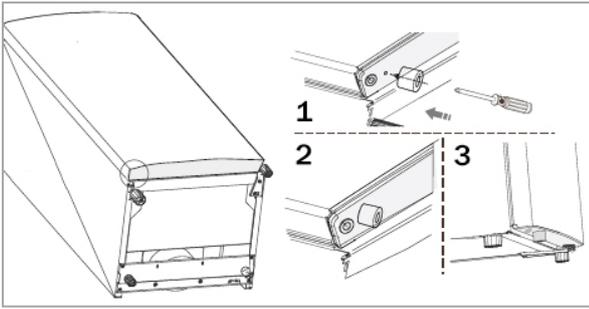
Tilt the appliance slightly back and block it in this position. Use the delivered screw to secure the supporting pad into the hole provided on the underside of the door.
